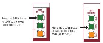
The operator will only keep track of up to 20 codes, then will start saving over the oldest codes as new codes occur.
